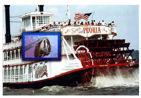
**Description:** One of the largest paddle wheel boats on the Mississippi River utilizes Ramsey chain to power the paddle wheel. Very high torque coupled with low speeds create a difficult scenario that many drives can not handle. Ramsey answers the call.
