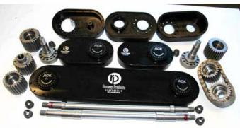
**Description:** Veteran motorcycle design team needed a reliable smooth running drive to achieve speeds in excess of 325 mph. Ramsey engineers worked closely with the customer to select, manufacture, and test chain and sprockets to prove concept. After weather prevented competition at the Bonneville Salt Flats, customer traveled to Australia to document their record speeds.
