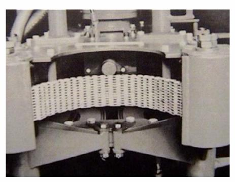
**Description:** Special chain developed to apply the high torque required to connect piping as oil rigs drill deeper for valuable oil reserves. Capable of transmitting up to 130,000 ft-lbs of torque. Used to grip, rotate, connect, or disconnect large piping.
