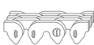
Insert short pin so convex pin surfaces are in contact
