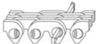
Insert longer pin through the chain
