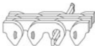
Insert longer pin through the chain
