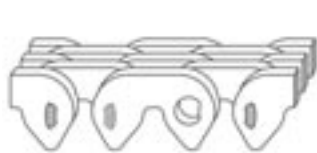
Bring the ends of the chain together so the holes are aligned
