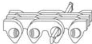
Insert longer pin through the chain
