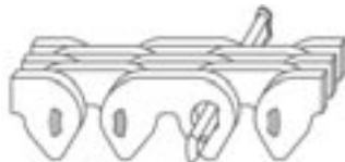
Insert longer pin through the chain
