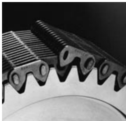
Symmetric chain lacing during connection
