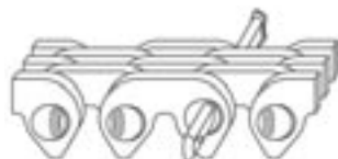
Insert longer pin through the chain
