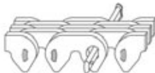
Insert longer pin through the chain
