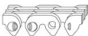
Bring the ends of the chain together so the holes are aligned
