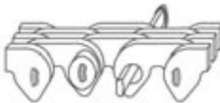
Insert longer pin through the chain.
