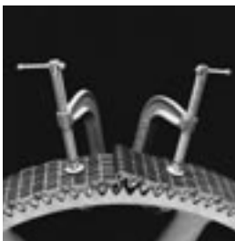
Chain clamped to the sprocket to simplify connection.
