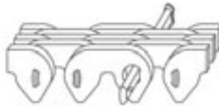
Insert longer pin through the chain.
