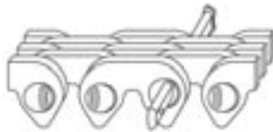
Insert longer pin through the chain.
