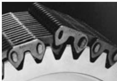
Symmetric chain lacing during connection
