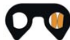
SC chain joint with "D" shaped pins
