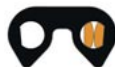
SC chain joint with "D" shaped pins
