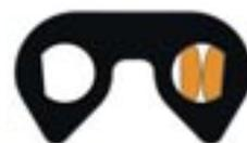
SC chain joint with "D" shaped pins
