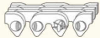
Put washer on long pin and install cotter or spirol roll pin
