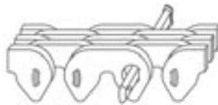
Insert longer pin through the chain.
