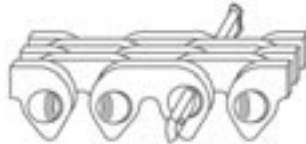
Insert longer pin through the chain.
