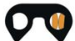
SC chain joint with "D" shaped pins
