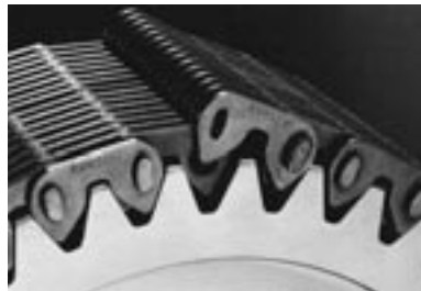
Symmetric chain lacing during connection
