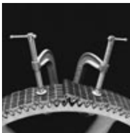
Chain clamped to the sprocket to simplify connection.
