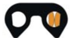
SC chain joint with "D" shaped pins
