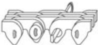
Insert longer pin through the chain.
