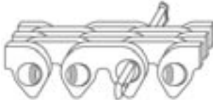
Insert longer pin through the chain.
