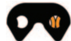
RPV and RP chain joint with "crescent" shaped pins
