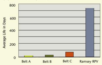
Results based on retrofitted 6 1/4" Ramsey take out arm in a high production bottling plant.
