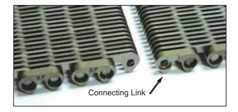
2) Slide the chain ends together so that the holes in the links are aligned.
