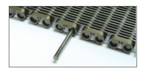
7) On the side of the chain with the connecting link use a small hammer to peen over the end of the connecting pin. Note: While peening the connecting pin it will be necessary to support the chain and prevent the connecting pin from coming out the back side of the chain.
