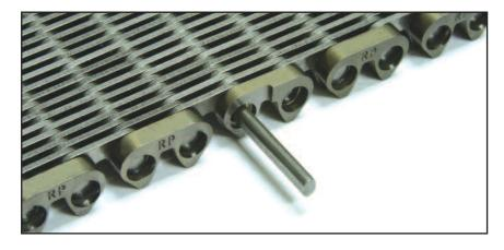
5) Locate the connecting pin that is headed on one end and softened on the other end.
