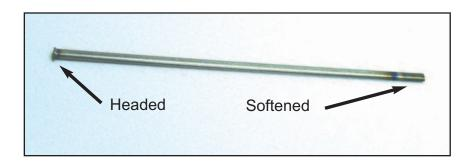
6) Move to the other side of the chain and insert the un-headed, softened end of the connecting pin into the chain.
