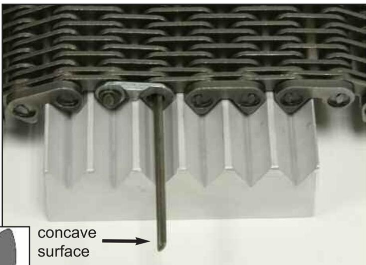
6) Insert the line up pin beside the short chain pin.
