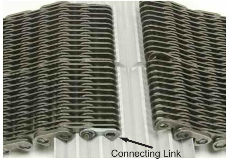
2) Slide the chain ends together so that the holes in the links are aligned.
