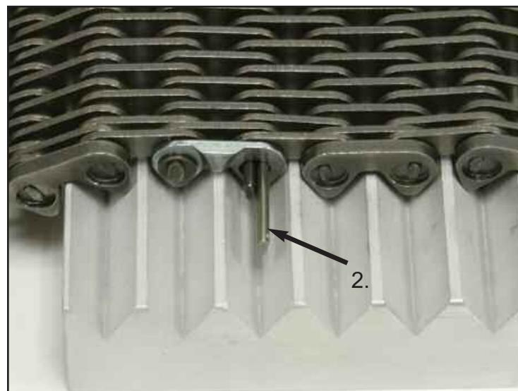
7) Insert the long chain pin with washer into the chain next to the short chain pin, pushing out the line up pin..
