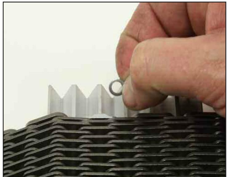
4) Insert the line up pin with tapered end first into the chain, passing through each link and each spacer.
