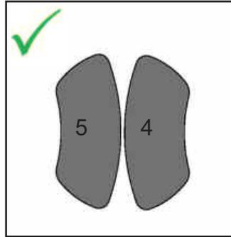
Make sure the concave surfaces on the long and short pin are opposite as shown here.
