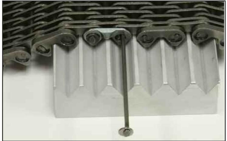
8) With the chain on its side, press the connecting washer on the end of the pin. Next, use a hammer to peen the end of the pin and the connection is complete.
