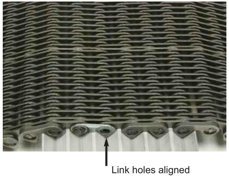
3) Insert spacers between the links in the joint being connected.
