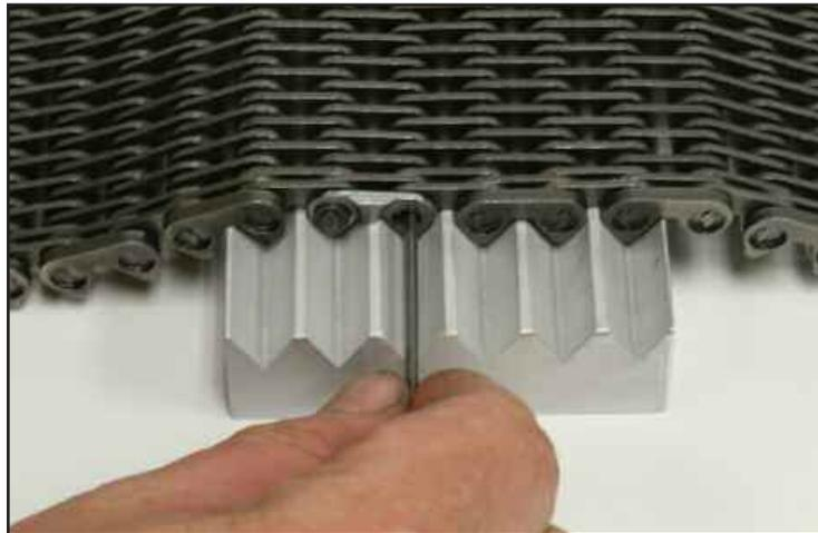
5) Insert the short chain pin into the chain, slowly pushing the line up pin out of the chain. The concave surface of the short pin should face the center of the connecting link.
