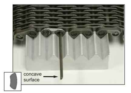
6) Insert the line up pin beside the short chain pin.
