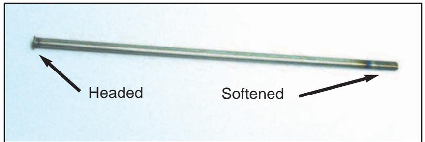
6) Move to the other side of the chain and insert the un-headed, softened end of the connecting pin into the chain.
