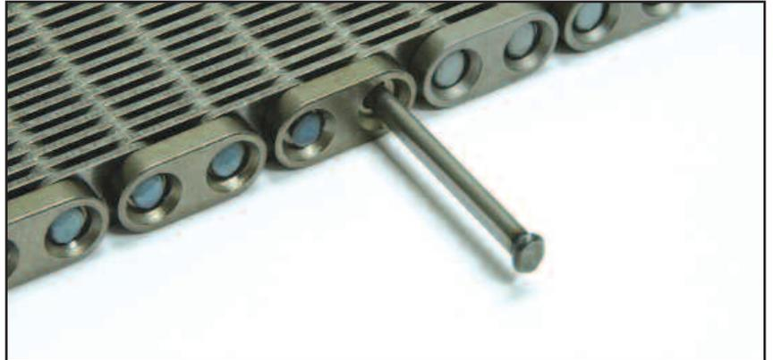
7) On the side of the chain with the connecting link use a small hammer to peen over the end of the connecting pin.
