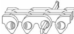
Insert longer pin through the chain.
