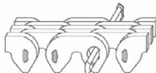
Insert longer pin through the chain.
