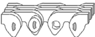
Bring the ends of the chain together so the holes are aligned
