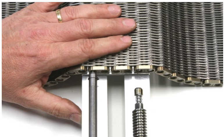
Quick and easy connection and disconnection of chain.
